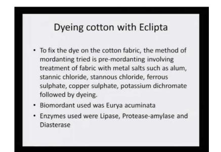
The Dyeing cotton with Eclipta extract to fix the dye on the cotton fabric, the method of mordanting tried is pre-mordanting involving treatment of fabric with metal salts such as alum, stannic acid, stannous chloride, stannic chloride, stannous chloride, ferrous sulphate, copper sulphate, potassium dichromate and then it is followed by dyeing.
