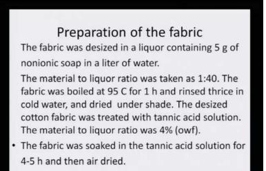
Now as what we know, that every fabric has to be treated before dyeing can be started. So, the fabric was desized in a liquor containing five gram of nonionic soap in a liter of water. The material to liquor ratio was taken as 1:40. The fabric was boiled at ninety five degrees for one hour and rinsed thrice in cold water, and dried under shade. The desized cotton fabric was rather discovered fabric was then treated with tannic acid solution.
