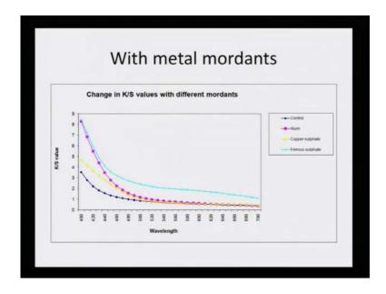
In order to make comparison, we also did and the same analysis with metal mordant. And metal mordants like alum, copper sulphate, ferrous sulphate and stannous and stannic chloride were all tried out, but this particular slide shows. The comparison between or the changing K by S of the control sample which has no mordant with alum, copper sulphate and ferrous sulphate.
