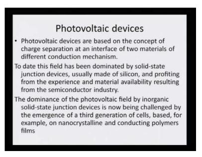
Today this field has been dominated by solid state junction devices specially made of silicon and profiting from the experience and material availability resulting from the semiconductor industry. So, it has been silicon and materials of silicones that have been develop which have been extensively use from making photovoltaic cells. Why because silicon has this very unique power of conduction and it has been found that it is an ideal material for these devices.
