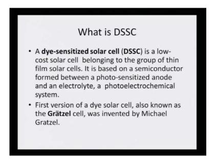
What is a dye-sensitized solar cell? A dye-sensitized solar cell is a low-cost solar cell belonging to the group of thin film solar cells. It is based on semiconductor formed
