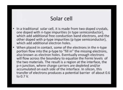
In a tradition solar cell, it is made from two doped crystal, one doped with n-type impurities - that is it is n-type semiconductor, which add additional free conduction band electrons, and the other doped with p-type impurities which is p-type semiconductor, which add additional electron holes. So, basically you are trying to conduct make more and more electrons conduct by using two different types of semiconductors, one is the n-type semiconductor and the other one is p-type semiconductor.
