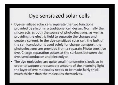
The Dye-sensitized solar cells: Dye-sensitized solar cells separate the two functions provided by silicon in a traditional cell design. Normally the silicon acts as both the source of photoelectrons, as well as providing the electrical field to separate the charges and create a current. In a dye sensitize solar cell the bulk of the semiconductor is used solely for the charge transport, the photoelectrons are provided from a separate photo sensitive dye.
