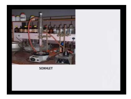
Now this is how the Soxhlet looks like, you see there is a round bottom flask, then there is a vessel where the plant material is wrapped up in filter paper, and there is a distillation head where the distillation takes place, and are almost eight hour this cycle goes on, till all the color actually collected in the round bottom flask, the round bottom flask is heated from beneath by a heating mantel. So, this is what this Soxhlet looks like.
