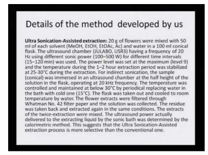
Details of this methods that was developed by us: I would like to share this, because this is one of the most innovative technology, Ultra sonication-Assisted extraction: Ideally 20 gram of flower were mixed with 50 ml of each solvent. Like one can use methanol, or ethanol, or ethyl acetate, or acetone and sometimes even water and in 100 ml conical flask it is just taken.
