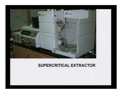
Now SUPERCRITICAL EXTRACTOR: This is how it looks and there is this liquefied carbon dioxide, which is popularly used for the extraction of the colorant. Sometimes some entertainers are added as a solvent like ethyl acetate, to facilitate the solubility of the colorant. Now because of the rarefaction of carbon dioxide, and liquid fraction of carbon dioxide, it adds on property to the liquid carbon dioxide, to be a good solvent.
