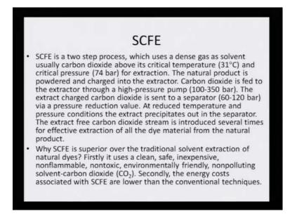
Supercritical fluid extraction or SCFE is a two step process, which uses a dense gas as a solvent usually carbon dioxide above its critical temperature that is 31 degree centigrade, and critical pressure which is 74 bar for extraction. The natural product is powdered and charged into the extractor. Carbon dioxide is fed to the extractor through a high-pressure pump that is working at 100-350 bars.
