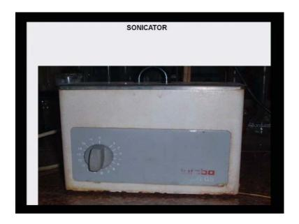
Now comes the Sonicator, now this is the machine which uses the ultra sound energy, and the ultra sound energy of 20 kilo hertz frequency, at voltage of about 50 can creates agitation which can be very good for extracting the colorant from the plant material.
