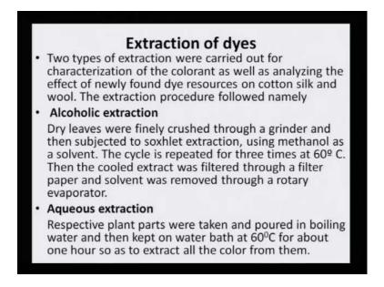
Therefore, extraction of dyes: Now can be you know summarize one can use Soxhlet method, one can use super critical method, one can use sub critical water, or one can use Sonicator method. But if I have to talk about extraction, then I will say that extraction of dyes are popularly done by two main solvents.
