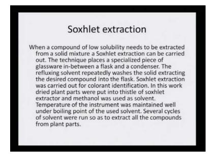
When a compound of low solubility needs to be extracted from a solid mixture a Soxhlet extraction can be carried out. So; that means, solid plant material cab be wrapped up, and with the help of appropriate solvent their solid extract ant can be or the dye can be extracted. The technique places a specialized piece of glassware in-between a flask and a condenser.
