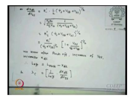
You can write this can give me a after differentiating it I Xdl verses VDS k one prime this other constants are took care it is psi s plus VSB to the power half one plus VDS upon psi s plus VSB to the power half we know after pinch off increase of VDS increase Xdl. So, the L effective L mask that is the actual channel length we keep minus the depletion layer and then we defined the channel length we entered lambda as one upon L
