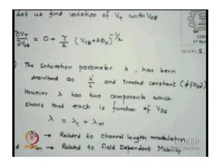
We will use later I just want to show that may vary the threshold variation is VSB which is gamma by 2 VSB plus 2 phi F to the power just differentiate. So, we see change in threshold voltage with subset bias; obviously, here is a minus value plus gamma by 2 VSB plus 2 phi F to the power minus half that half will come and minus will appear due to differential.
