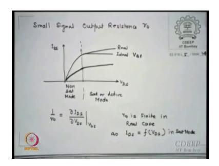
If you see yeah ids VDS characteristics in saturation this is my ideal this is my real the slope as I said may not be constant so, but for a one VDS I may say it is one value now I may find r 0 as delta ids by delta VDS slope of this characteristics r 0 is finite in real case because there is a slope and ids is a function of VDS inside that is what one plus lambda VDS term we derived ok.
