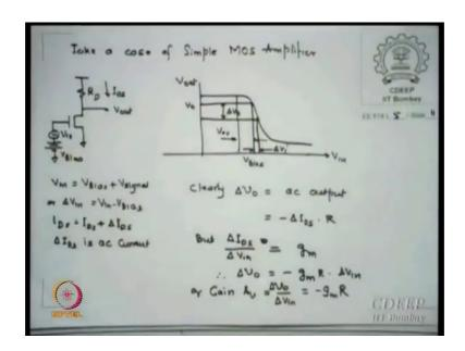
And right now this node is rd I start looking like that the input V in is V bias plus V signal. So, change in delta V in which is signal is V in minus V bias we always define small id capital Ds is equal to small ids which is the ac current of variant current time varying and this is dc this is how small signal values are expanded delta ids is the ac current. So, if I bias this is my MOS vi for an amplifier VA vi characteristics.
