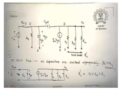
This is only a normal nature systems, which many years we have been using so Vinay Mizuki having drawn that figure I can make equivalent circuit of this I have an input source which is AC signal small signal. This is the source impedance R signal then there is a RG which is the bias resistance which may be due to the RG1 or RG2 parallel combinations then of course.
