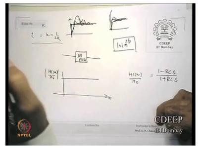
This is not the exact one what is it trying to tell you this transfer function (FL) said every frequency you get flat is that correct. However even if you see this function (FL) phase can vary depending on RC values phase can vary from 0 to 180 degree, so whenever the transfer function filters you create and you want a particular phase at the output between in and out then you connect the last stage of your filter can be all pass filter with proper phase requirements is that clear to you.
