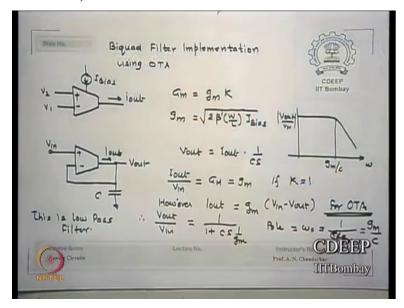
This is another which is an integrated circuit filter (FL) what is the difference between operational amplifier and operational transconductance amplifier (FL) see if I were an amplifier whose output current is controlled by input signal then I have a operational transconductance
