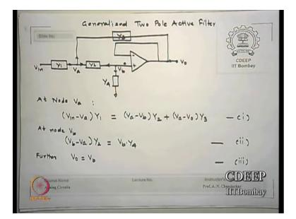
So, I have now suggest you here is a circuit active filter which is a generalized to coal filter how much how many what you mean by two poles how many capacitor RC's it should be 2 RC's system okay. This is generalized why I say generalize what does that mean generalize means, all four filter should be clear can be created out of this is that clear generalized I never said it is low pass, high pass, band pass.
