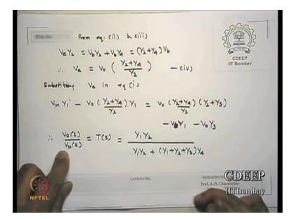
I did just look at the final transfer function you write and verify V0 S by Vin S which is my; either you write PS or you can also write HS whichever way you are writing either T is the transfer function okay. Normally I have been using H as the transfer function but I do not know from wherever earlier and there was a T, so I use T. So, maybe your colleges, so I get Y1 Y2 upon Y1 Y2 this kind of function.
