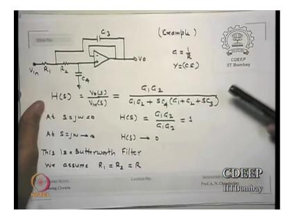
Now in this I create the first Y1 Y2 I put it as R1 R2 and this Y3 I4 I put as two capacitors in our case G is 1 upon R and Y is CS okay B rather not but these are Y only, this is capacitance. So, CS is the admittance of that and conductance of this is 1 upon R1 and 1 upon R2, this is the expression I just got further transfer function G1 G2 upon G1 + G2 + SC 4 G1 G2 SC 3. So, now you look at it at S = 0, what is the value of HS. (FL)
