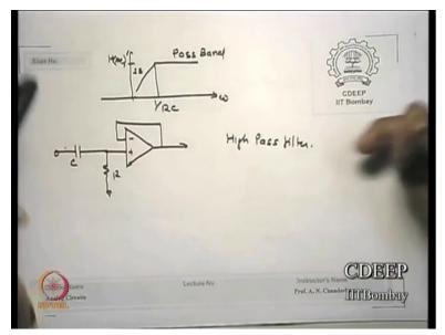
So, initially what could occur you can see from here 20 DB, 0 means 20 DB per decade rise start rising okay. At the pole what is the fall should be -20 DB but what is it rising already with 0, +20 DB. So, at this point onwards 20 - 20 is 0 DB gain becomes our output function becomes constant is that high pass requirement at frequency above 1 upon RC, I want transfer function to our unity value all no attenuation it just passes out inputs is that correct.
