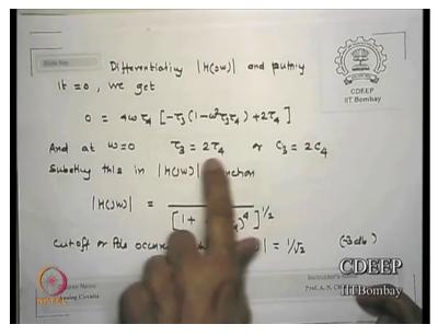
Okay, I can get a condition tau 3 is tau T4 and C3 is 2C4 (FL) is that one clear. I differentiated that below that cutoff and I say at this point if I want no ripple then what should happen if I meet these conditions then I would say I am going to have a maximally flat situation is that correct. (FL) We can remove by actually choice off proper tau's and C's is that clear, all other C's, C3 should be twice of C4 in our case.
