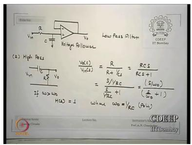
So, basically active low pass filter I really could be a RC circuit as I just now do followed by a voltage follower is that kind of followed by a voltage follower. So, whatever is the voltages here will be transferred here because a voltage follower. So, this is the easiest way of making a low pass filter we are not seen as transfer function so far. So, we do not know whether it is going closer to ideal but this should do as a low pass filter with an active device.
