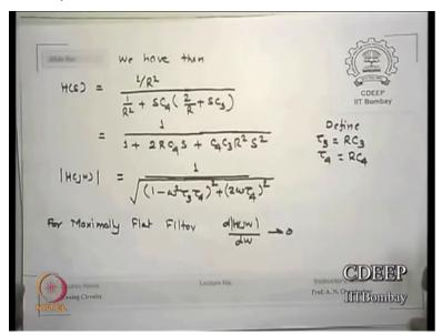
So, I wrote the transfer function as it is (FL) is it clear but I just substitute G 1 upon R and twice GS and I get this function if I manipulate it better and I give a definition that tau3 is RC3 and let us assume R's are equal. My assumption is R's are equal but I never said C's are equal, R's are equal but see why I do not want to make C is equal because then the time there will same poles will come. So, I okay there are two different poles one is greater RC3 the other related to RC4.
