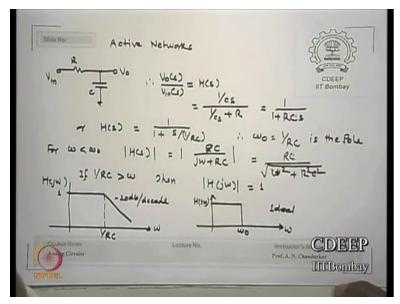
We are done this earlier is well, if you are a RC network 1R and 1C, if I take a transfer function of this V0 by Vin is 1 upon CS upon 1 upon CS + R which is 1 + RCS or it can be written as 1 upon 11 by RC, if I define a frequency cutoff frequency as 1 upon RC this is nothing but 1 upon S by Omega0. What does that mean there is a pole in negative half2 - Omega 0 and if I plot the Bode plot therefore at this the gain will start falling okay.
