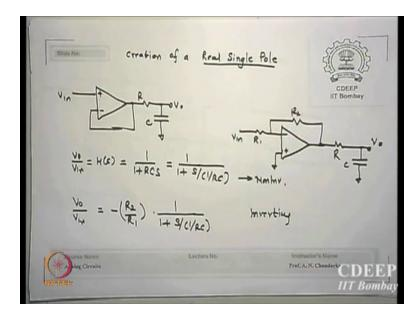
Okay, (FL) is that current real pole requirement. So, here is a single real pole (FL) RC this the filter input is not loading input is coming here with high impedance on that so it is not getting loaded by this (FL) if you want a gain fine if you do not want to put R2 = R1 so that will become 1 upon s by 1 upon R thing with a - sign is that clear choice have RR yours.
