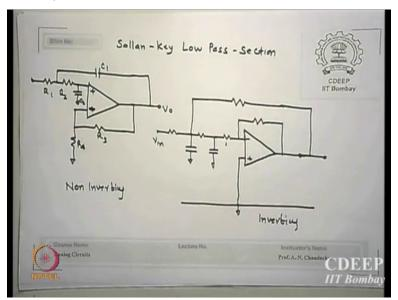
This is called Sallan and Key Low Pass section okay, now this words section is clear. How many Poles this is going to realize each of them inverting and non-inverting two poles (FL) is that clear the constants which you are derived expression I mean you have got from functions had to be now implemented through R1 C1, R2 C2 values but that is normally taken higher you can see now your gain is now reduced. (FL)
