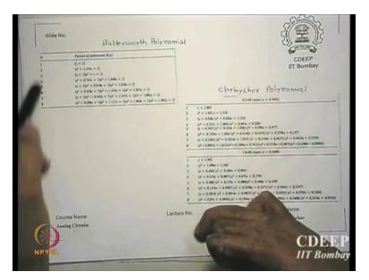
Here is I just copied it the Xerox, this is the order of polynomial Butterworth polynomial 1, 2, 3, 4, 5, 6, 7, 8, this is normalized polynomial BNS (FL) I am realizing in butter well it S + 1 that is a pole, S + 1, if N = 2; I am realizing S square + root 2 S + 1 okay, if N = 3 it is S + 1 times S square + S + 1, if N is 4 S 2S squared terms will appear 4 means (FL) so 4 poles is that correct. These are number of poles, 5 means S + 1 into 2S square bracketed term is that correct.
