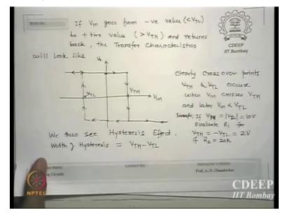
If I am going from -VL to -V in + when the output was high then what will happen it will switch over at this value VTH. However if I am at VL and I am reducing V in it did not switch on here why because now the value of switches at VTL - of that time is that clear. When I went from - V2 + V in as we became crossing that V + value the step change is high to low it went through okay. (FL)
