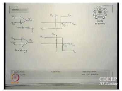
We will last discussing about comparators and we did say that if V in is larger than the reference are smaller than the reference output will be correspondingly + or - and two circuits which may be used one is inverting kind the other is non-inverting kind may have a characteristic shown here. If it is a non-inverting for being less than 0 are smaller than V reference you have V low. At V reference when it crosses it will jump to high value which is VH.
