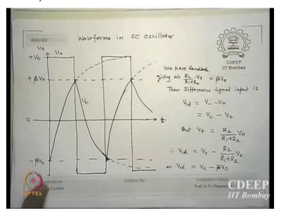
Before they come here okay (FL) before we say if in this circuit what is being fed back (FL) which is nothing but I2 upon R1 + R2 times V0 (FL) is that okay (FL) is that okay beta is sink feedback factor voltage received from the voltage V0 (FL) so, this is the voltage which is V + across RC0 V + is that okay (FL) - beta V0, is that correct two values of V + I can attain either + beta V0, V0 is positive. If V0 is negative - beta V is that okay.
