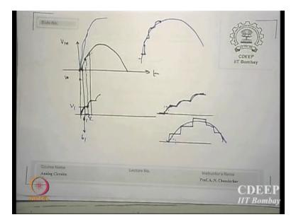
This is what essentially I am now seeing example (FL) time varying these are the instances when I am actually going to turn on the switch (FL) Vin pass as it is please remember ideal switch (FL) which in reality there is an issue there but right now so if Vin is here it will start charging to that value it will output will follow V in charging the capacitor (FL) is that okay so it charges to some value which is so V1 which after them. (FL)
