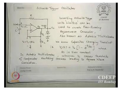
The circuit which I am interested in is those oscillators why am I did all that because to understand the operation of this. I thought you should first learn the Schmitt itself is that point clear. Otherwise for this circuit I could have started here and say this is how it happens but I thought it is not fair let us say what is Schmidt and then use Schmitt trigger to create an oscillator. Please take a circuit okay. (FL)
