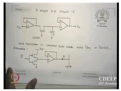
Second Circuit has is a discrete value or some other circuit whose input impedance is not very high which like at this transistor does not have I must always feed input to this through what a buffer okay follower. (FL) Transistor is turned on if Vin is higher than VT less than it is off. So, I had a control signal which goes from 0 and 1 higher or lower value and allows input to charge the capacitor and hold it. (FL)
