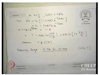
So, t = T by 2 VC T is beta V0 so beta V0 (FL) 2RC Ln 1 + beta upon 1 - beta which is 2RCLby R1 + 2 R 2 by R1 (FL) is that oscillation clear to you because V0 changes the state beta V0 goes from - beta V0 + V2 which is about threshold values. So, capacitor charges to 1 discharges to other so the output spring from high to 1 node 1 or V0 (FL) VZ + VD this is - VZ + VD is that clear. (FL) The period of this Smith oscillator is to RC Ln 1 + 2 R2 by R1, R2 by R1 can a feedback ratio.
