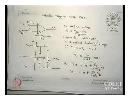
So, that is advantage of Schmitt circuits (FL) I will just show you I instead of you know this putting to be there for me this is a inverting kind (FL) if I do the same analysis once again the transfer characteristics will now move away from that point okay by so much as V reference point by ratio of; there is a potential called VS which is the half way switching voltage as we call VTL + VTH- VTL by 2 which is again R2 upon R1 times R2 (FL)
