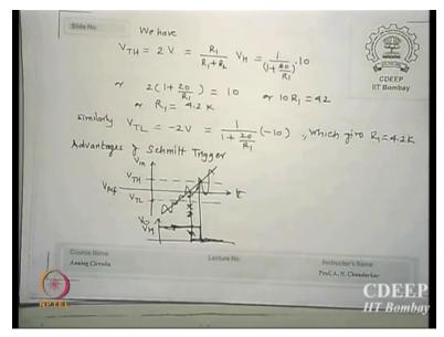
Either use VH or use a VT h or use VTL either of them VTH is R1 upon R1 + R2 times VH that is given to you 2 volt. (FL) So, R1 upon R1 times VH is 1 upon 20 by R1 into 10 this gives me a value of 4.2k, if I use -2 volt (FL) either use VTL or will use VT as longer they are saying it does not matter, it does not. What is the design we say okay (FL) so, it should be 4.2k is that clear that is how you actually will hook up the circuit.
