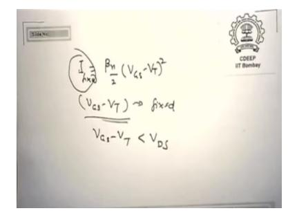
Now so if I is fixed Vgs-VT is fixed we make i sufficiently such that Vrs-VT is always less than VDS choice of i is such that Vgs-VT is smaller than VD s so when I fixed active load which is current source I am actually biasing the device in saturation the choice of I is mine is that correct choice of I is mine which will fix my bias for any transistor is that correct same current is passing in and one same current is passing in M2.
