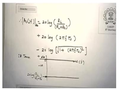
So I say at F=1 upon 2 pi hours please take the frequency F=2 pi tau s what is the value of bracketed term 2 pi F tau s is how much 1 how much is value of log 1 0 log 1 is 0 so it is at 0 dB is that clear F is equal-1 upon 2 pi hours if that is equal to 1 so at F is equal to this frequency the gain is 0 dB this second term only I am saying not the net one only second term if I multiply it by ten frequency that is if this becomes 10 upon 2 pi tau s okay.
