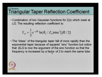
Now derivation of the triangular paper function is not that simple it is actually the combination of two Gaussian functions, in that case the Gamma in value is given like this which is actually proportional to square of the sync function. So impedance that we can derive from the triangular taper function or this triangular taper is that the frequency...
