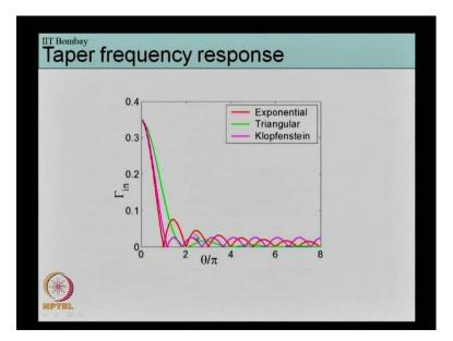
...if we go back to the slide that this green line represents the input reflection coefficient of triangular taper and this red line represents the input reflection coefficient of exponential taper. And we see that the frequency of the ripples for the triangular taper is actually half that of the
