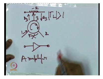
One is if you say this is your circulator and you connect a negative resistance to say port 3, port 2. Now negative resistance will always cause input say if this is my say B3 that is entering this negative resistance, then A3 the wave incident at port 3 but reflected from the load will be at the magnitude of this wave will actually be greater than the magnitude of B3 because Gamma-L magnitude will be greater than 1.
