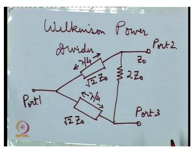
So, the circuit for this Wilkinson power divider is like this. The circuit is like this and any power entering port 1 will be equally divided between port 2 and port 3 but no component of power entering port 2 will appear at port 3.
