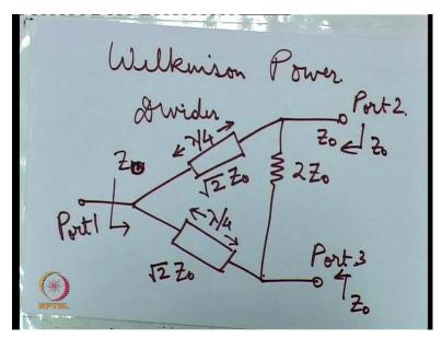
Now you can verify that the input impedance is Zin Z0 for all the ports. The methods have been shown in the slides associated with this analysis methods have been shown in the slides associated with this lecture. The S parameter matrix of this Wilkinson power divider can be given by this equation.
