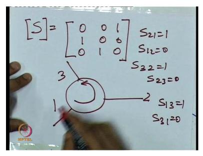
the final S parameter matrix that I get for this circulator can be given as... The symbol of a circulator is like this, this is port 3, this is port 1, this is port 2 we use and arrow to show the direction in which power transfer is allowed, so in this case, power as also seen from this S parameter matrix, we see that S 21 equal to1 but S21 equal to 0.
