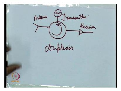
And one other use of circulator is what is known as a shared antenna. So, a shared antenna, you know in communication we have to use the same antenna often use the same antenna for both the transmitter as well as the receiver but then to do that, we have to allocate different timeslots for the transmitter and the receiver.
