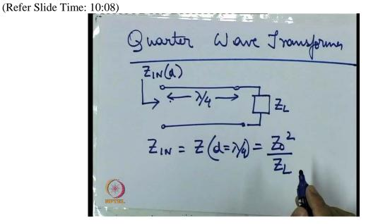
For quarter wave Transformer is a transmission line which is quarter wavelength long i.e. lambda/for long. It is also terminated by a load ZL. Now, in place of Zd I can also write this as Zind. So Zin will be equal to Zd equal to lambda/4 and this comes out to using the equation that I just gave if we put in the equation that I had previously stated that if this equation
