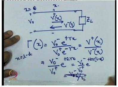
So once again if we have our transmission line with a load ZL connected like this and suppose the voltage as I said there are 2 concepts, one is V+ and V-then the reflection coefficient at a particular length x is given by V- or E+ gama into upon (V+-gama x).
