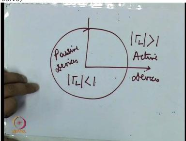
So we can write this as suppose this is a unit circle, the circle have been unit radius and within the circle, we have gamma L modulus lesser than 1 and outside the circle, we have gamma L modulus greater than1. So this corresponds to all active devices and this corresponds to all passive devices. In the same way that we obtained the curve from Z value, we should also be able to get the curve, Smith chart form the Y values and such a Smith chart is called as Y Smith chart.
