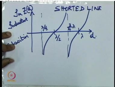
So we can see a shorted transmission line can take on both positive values as well as negative values for different values of d. For example, when d is equal to 0, it has a 0. So it is like a short. When d is between lambda/2 and 3lambda/4, it is positive. Zd is positive for a shorted line. So this is for a shorted line. Zd is positive. So it acts as an inductor. When d is between lambda/4 and lambda/2, Zd is negative and hence the shorted transmission line acts as capacitor. A special
