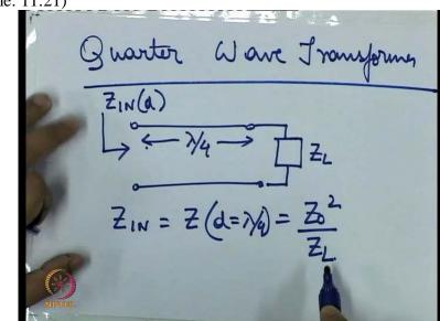
So what we see is that the input impedance is proportional to the inverse of the load impedance. If the load impedance ZL shorted, input impedance will appear to be open. If the load is open, the input will appear to be shorted.
