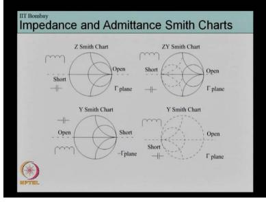
So if we can go back to the slides the monitor for a moment, these are the various configurations of the impedance and admittance Smith charts. Say this is our impedance Smith chart, then the top half we will have inductive i.e for the top half, the reactance X will be positive and for the bottom half, reactance X will be negative.
