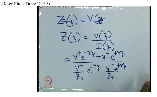
The impedance at any point Z or X's whatever. We can take X also in place of Z is given Z of small is equal to V of Z upon I of Z. If I write the voltage and current relationship at Z, that is...now this can be simplified to this relationship.
