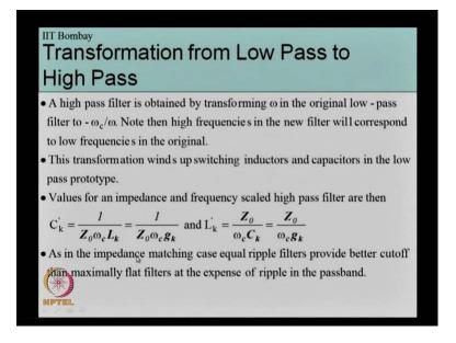
In that case the inductances will be converted to capacitances and capacitances will be converted to inductances as given by this value. So, here GK are the lowpass prototype and CK are the final values for the high pass prototypes with certain Z0 and omega C, they need not be equal to 1 ohms and 1 radians per second.
