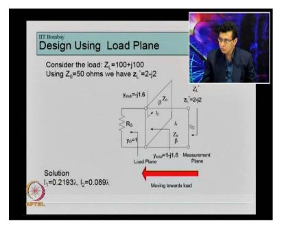
The 1<sup>st</sup> thing we note that as I had mentioned that when we go along a transmission line, if this is supposed the implementation that we want, that is 1<sup>st</sup> length of the transmission line followed by a shorted stub. When we move along a transmission section of a transmission line, the magnitude of the reflection coefficient along the transmission line remains constant.
