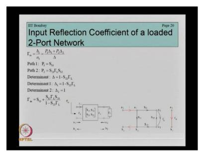
Now then coming back to over 2 port circuit as shown here, the path 1 gain is simply S1, the gain of this path, S1. If we go from A1 to B1 along this path, it is S11, the path gain of path 2, that is starting from A1, going straight, turning and then returning to B1 is S21 multiplied by gamma L multiplied by S12. And then what is delta, how many loops do we have? We have only one loop.
