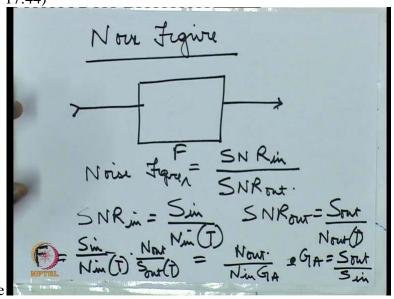
Suppose we have a 2 port network. That is say an input signal and an output signal. The noise figure is defined as SNR in upon SNR out. No it is not SNR out upon SNR in. It is SNR in upon SNR out unlike other terms. Unlike gain term where you always have output in the numerator
