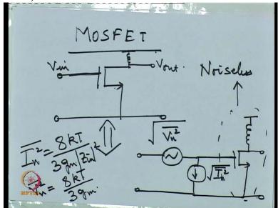
Let us see a simple MOSFET which is an active device and has some noise associated with it. In fact, a simple MOSFET has a circuit like this. Now the equivalent noise circuit for this MOSFET can be given like this. This is noise less and value of this IN square is given by the value of this VN square is given by. And related term that is often associated with 2 port networks is what is known as a noise figure. Now let us see what does the term, noise figure mean? (Refer Slide Time: 17:44)
