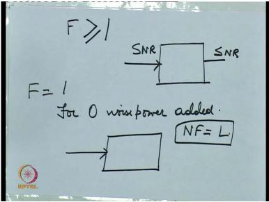
Now some of the properties of noise figure are that this F is always greater than or equal to 1. It cannot be less than one because in any 2 port network, the SNR of the input will always be greater or at best equal to the SNR of the output. They will be always sent out noise contributed by the network. Hence the signal quality will either remain the same or will be a little bit degraded than the output. Hence, SNR in can be never less than SNR out. Therefore F will always
