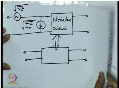
Now for 2 port network like this so for 2 port circuits, this is a noisy 2 port circuit various noise elements present. From that if we have to go to a noise less circuit, then we make a transformation like this. And how you know the derivation of the values of this VN and IN is given in appendix L of the book by Gonzales. Please go through it.
