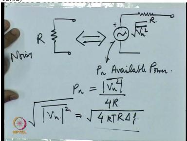
And this available power value is given by PN is equal to VN square by 4R from which this noise voltage value can be found out to be 4KTR delta X. So this is the equivalent noise voltage
