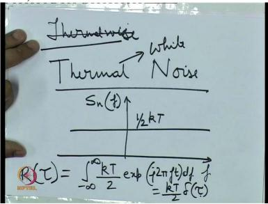
One of them is what is known as a thermal noise. Thermal noise is a distribution like this. Autocorrelation function for this thermal noise is given by this equation.
