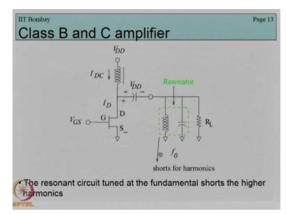
In Class B instead of just an RL we now have a resonator with resonant frequency of F 0 connected in shunt with the load RL. Remember that this ensures that the total DC current consumed from the source V D is constant.
