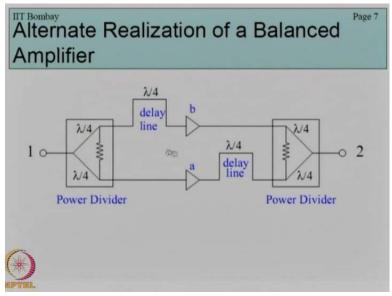
Now here what you have is a power divider recall we have covered power divider, 2 identical power dividers, 2 identical delay lines and 2 identical amplifiers.
