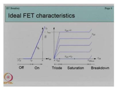
So this is a MOSFET whose drain current versus gate source voltage relationship is like this and whose drain current versus V D S that is drain source.
