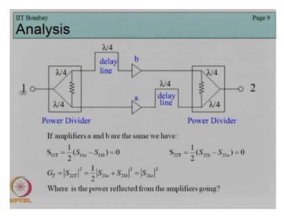
What happens is that here also reflections take place, but instead of coming back to the Port 1 or Port 2, they are kind of synced or wasted away in these in this resistant that is present in the power device, so in this but module will covered a number of topics especially on frequency compensation DC bias and also power and also broad band impedance matching as well as broadband gain matching.
