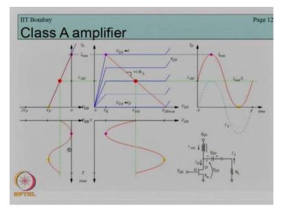
First of all, note that because it is operating for the entire region that is the transistor is always on, our input will have to be in that region of the I D versus V G S characteristics where the entire 360 degree can be accommodated.
