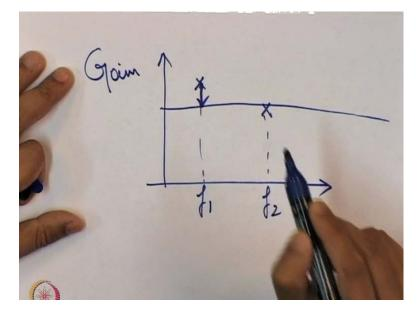
At a different frequency I have this as the gain, so how can I keep my gain constant? One way is to simply use the filter with a very broadband and bring this gain down, so that it matches with the gain of this one at this frequency. This way we are compensating, making the forcefully making the gain same over the entire range. Or you know so to do this what can we do in a so we have a higher gain at a different frequency.
