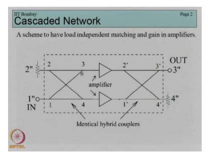
What is happening as I said in all the reflected waves are get added up at Port 2 dash, so there is a load match load connected at this Port 2 double dash where kind of the where the reflected powers are synced or wasted away.
