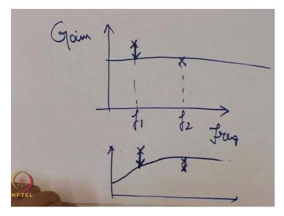
So we don't want to reduce the gain here, but we want to reduce the gain here. So if we choose a filter with a characteristics like this, what will happen is because the gain is low over here, this gain the inherent gain at a particular frequency will be brought down while the gain at the other frequency when we don't want it to be attenuated will continue remaining the same. Some example of yet another example if we take if we go to the slides on... if we go to the slides on the on the monitor.
