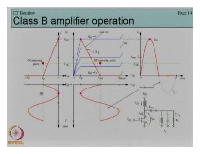
Therefore my input is now like this. See only the half cycle, only doing this life-cycle it lays the... The input lies in the conducting region of the transistor. Now because it is now conducting only for the half cycle, not how I D changes. I D is now like this, a single half cycle and then it stops. But what about my V D V D D S my V D S? V D S on the other hand continues to be a sinusoid.
