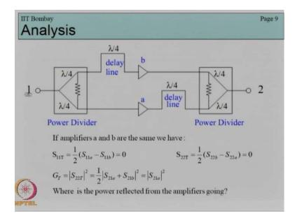
That is the total input reflection coefficient and output reflection coefficient will always be zero. Not when I say always I I you might be thinking I mean infinite bandwidth, it is not in finite but a very broadband kind of. Provided of course we have perfect matching between the amplifiers, perfect matching between the power dividers and perfect matching between the delay lines.
