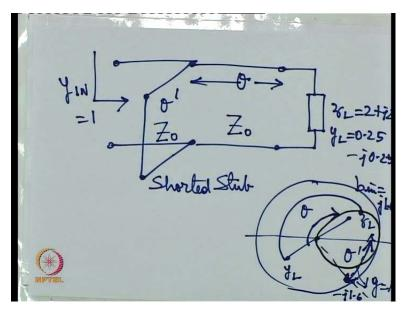
So just to summarize the whole process, I have a ZL. This corresponds to YL equal to .25 minus J .25. First I connect a length of transmission line corresponding to theta. Then I add a shorted stub of length theta length and I get Y in equal to 1. On a Smith Chart this would look like this.
