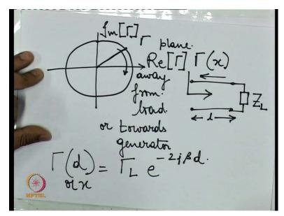
So as you know, as we discussed in the previous class, the Smith Chart originates from the concept of the reflection coefficient. If I can just redraw that figure...so this is the gamma plane and as we go away...so if this is the representation of a transmission line with a load ZL connected then, and say this is a transmission line of some length L, then as we are going away from the load, our phase angle decreases and that's why we are going in a clockwise direction.
