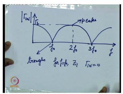
If I plot this expression, the kind of graph that I get is like this. So there are troughs and then there are peaks. For F equal to F0 okay, the input impedance is Z1, hence gamma in is equal to
