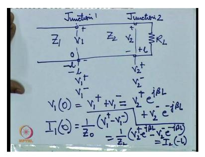
So if we can go back to our figure, let me draw a fresh figure. So we have one transmission line with characteristic impedance z1, & another with characteristic impedance z2. V2+ is the incident wave at junction 2 & v2 - is the reflected wave at junction 2. V1+ is the incident wave at junction 1, v1- is the reflected wave at junction 1.
