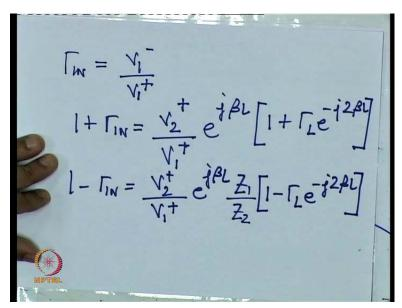
So i1 of 0 is i2 of -L with appropriate coordinate transformations & then gamma in, which is defined as d1- upon d1+, that with this definition, we can write 1+ gamma in equal to v2+ upon v1+. So this is the 2 expressions that we can find for 1+ gamma in & 1-gamma in.
