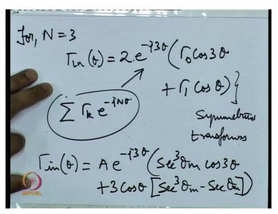
So these are the expansions and what we say N equals to 3, gamma in theta using these expressions that I had derived in the previous slide, you can write gamma in theta is equal to, this is the expansion from the earlier expansion that we had derived, this when expanded for third order we get like this, ah this is of course only true for symmetrical transformers and using the Chebyshev expansion that we just saw... Gamma in theta can be given like this.
