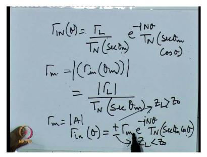
And we know that this positive sign is for ZL greater than Z0 that is when gamma L is positive and this negative sign is for ZL lesser than Z0, that is when gamma L is negative, now how do from here to the design, the nice expressions that we have derived for our binomial transformer, how do we do that.
