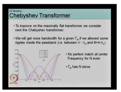
To answer that question if we can go back to the monitor slides for a moment. Ah see these are the Chebyshev polynomial expansions for various order, if the red one is for N equal to one, then this N equal to 1 polynomial is very similar to the binomial expansion then the blue one represents N equal to 2 black one N equal to 3 and violet or purple one represents N equal to 4 Chebyshev polynomial.
