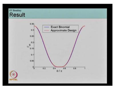
The other thing is when we do this design we see that there is a slight mismatch between the exact binomial formula and this design that we have implemented on the circuit and mismatch is because...
