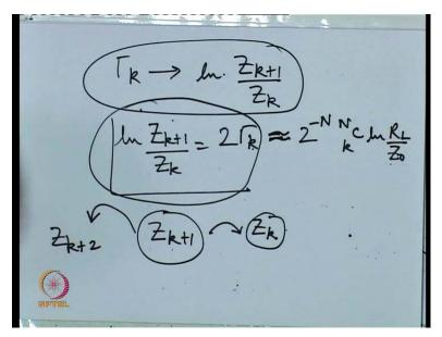
if we can come back to the written slide for a moment is because of this approximation, this logarithmic approximation that we give, because of this, there is a slight mismatch, so that was all about design using the binomial transformer.
