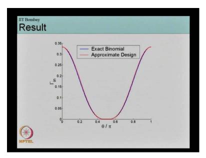
Here is a P section binomial transformer the input reflection coefficient that we design, we see that there is a slight, you there is slight mismatch between the exact binomial function represented by the blue line and this red line representing what we actually implemented.
