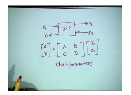
The set  $[X_1, Y_1]$  is expressed in terms of the set  $[Y_2, X_2]$ . In similarity with analog two ports, the corresponding parameters are called the chain parameters and denoted by ABCD. Why are they called chain parameters? It is because if you have a chain of D2Ps, then the overall ABCD matrix of the cascade shall be the multiplication of the individual ABCD matrices, written in the same order as they are cascaded.
