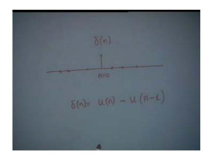
$\delta(n)$  is simply one signal of amplitude 1 at n = 0 and the rest all are 0. Obviously, for  $\delta(n)$ , you subtract from u(n) all that occurs to the right of n = 0, which is simply u(n - 1). Therefore  $\delta(n)$  can be replaced by u(n) – u(n – 1). I think our time has come to an end and therefore we will stop here today.
