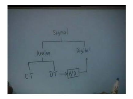
We also said that basically there are two kinds of signals: analog and digital. Analog can be continuous time (CT) or discrete time (DT). A discrete time signal is not a digital signal; a discrete time signal is one in which the amplitude is a continuum, and not discretized. On the
