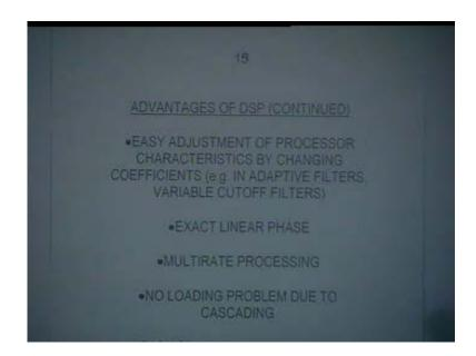
You simply change a number which is one of the coefficients and then you get a different characteristic. This is required in adaptive filters or variable cutoff filters.
