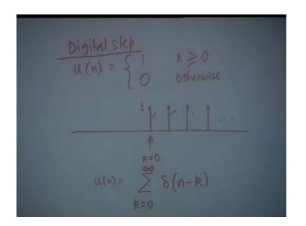
A combination of such impulse functions give rise to a digital unit step u(n); u(n) is a signal which is 1 for n greater than or equal to 0 and 0 otherwise. Obviously u(n) can be written in terms of  $\delta(n)$ ; it is summation of  $\delta(n-k)$ , k going from 0 to infinity.  $\delta(n-1)$  describes an impulse with one sample delay,  $\delta(n-2)$  is an impulse with two samples delay, and so on. So u(n) is very simply related to  $\delta(n - k)$ .  $\delta(n)$  can also be related to u(n).
