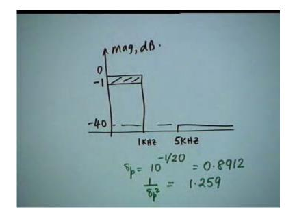
As in the previous example, let the stop band start from 5 kHz and let the minimum attenuation be – 40 decibels. So the first thing you do is to find out  $\delta p$  and  $\delta s$ . Here  $\delta p = 10^{-1/20}$  and that comes out as 0.8912. What we need is  $1/\delta p^2$ , which calculates out as 1.259.
