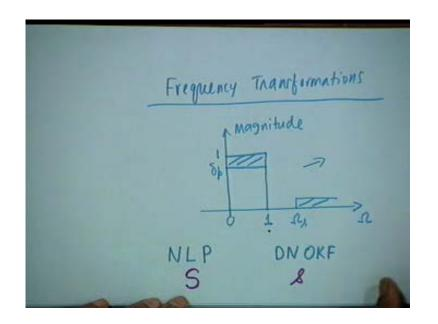
We next consider frequency transformation in analog filters. What we wish to do is to transform a normalized low pass filter with cutoff at 1 radian/sec into other kinds of filters in which the cutoff frequency is  $\Omega_p$  radian/sec. This cutoff frequency could be 3dB frequency for Butterworth or it could be 1dB frequency for a Butterworth, or it could be .5d B for Chebyshev.
