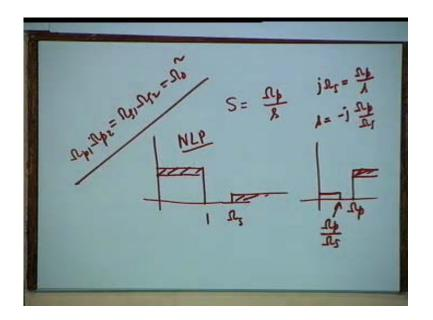
Do you understand the steps? The steps are: from the specifications of the desired filter, you go to specs of normalized low-pass filter (NLPF); then design the (NLPF) and use transformation to get the required H(s).
