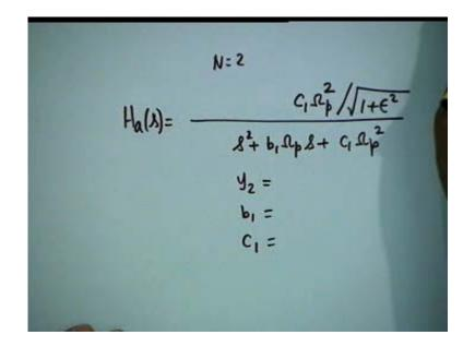
If N = 2 then you can immediately write  $H_a(s) = [C_1 \Omega_p^2 / \sqrt{(1 + \epsilon^2)}] / (s^2 + b_1 \Omega_p s + C_1 \Omega_p^2)$ . Here  $\Omega_p = 2\pi (10)^3$  radians/sec. N is even and therefore you must have the factor  $[1/\sqrt{(1 + \epsilon^2)}]$  in the numerator. For finding out  $b_1$  and  $C_1$  you have to find out  $y_2$  first.
