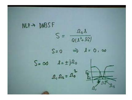
This is another way of saying that at the same attenuation the two frequencies are geometrically symmetrical with respect to  $\Omega_0$ .
