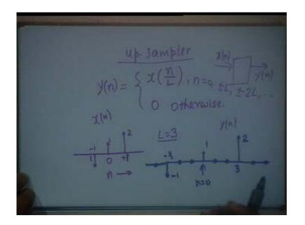
In up sampling, the relationship between y(n) and x(n) is y(n) = x(n/L). Obviously y(n) will exist when n is an integral multiple of L. Digital signal exists only when argument is an integer, positive or negative, so y(n) exists for  $n = 0, \pm L, \pm 2L$ , and so on, and it is 0 otherwise.
