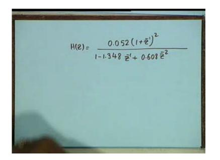
The magnitude response of this transfer function, as shown in the next figure, does not start from 0.8; it is slightly raised. The maximum also is not 1. This happens because we computed only up to three places of decimal.
