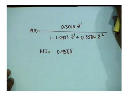
You should keep as many digits as possible because the filter design is extremely sensitive to quantization or to truncation errors. For example, the dc gain H(1) should have been 1, but here it is 0.9568 which is quite a substantial deviation, more than 4 % from the unity value.
