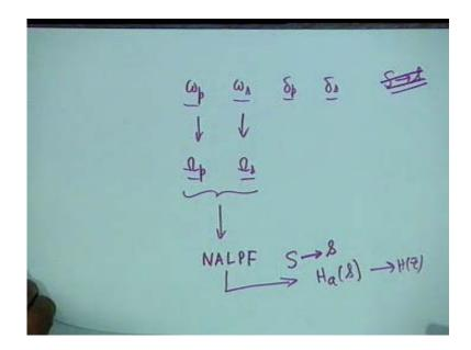
In multi-band pass filter,  $\delta_p$  may be different in different pass bands; then you choose the minimum tolerance. But if it is a stiffer requirement, then you may have to use a different kind of transformation from S to s; simple band pass or band stop transformation may not suffice. You
