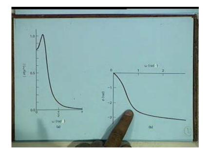
This is the effect of truncation error; even up to three places of decimal is not good enough. As far as phase is concerned, it is approximately linear up to about 0.8; radians and then the nonlinearity starts. So if your signal processing or pass band is confined to this limit, then you can be reasonably certain that there will be no delay distortion. If you go beyond this then you have to use an all pass filter for equalization.
