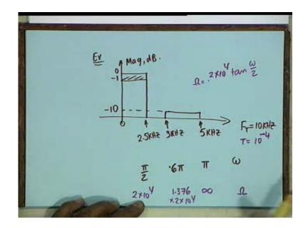
Beyond 3 kilo Hertz, the magnitude response must be down by at least 10 dB. One could expect that this would be satisfied by a sufficiently low order filter but you must also see that the transition band is pretty narrow. The stopband end is 5 kilo Hertz which means that the sampling frequency,  $F_T$  must be 10 kilo Hertz.
