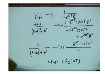
For a simple pole in H<sub>a</sub>(s), the term  $1/(s - p_i)$  goes to  $T/(1 - e^{p_i T} z^{-1})$ .
