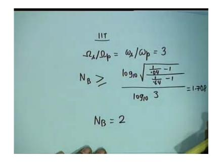
We still continue to use Butterworth. Here calculation gives  $N_B \ge 1.708$  and therefore  $N_B$  is still = 2. In order to design a Butterworth filter, you also require the value of the 3 dB cutoff frequency  $\Omega_c$ . here it is  $(\Omega_p/T)/(1/0.64 - 1)^{1/4}$  (instead of the tangent) and this calculates out as 0.7255/T.
