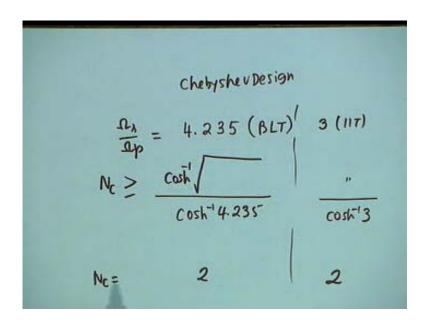
With  $N_c = 2$ , your transfer function will have a multiplication by T in IIT, not in BLT. The transfer function  $H_a(s)$  have a multiplying factor  $1/\sqrt{(1 + \epsilon^2)}$  for  $H_a(0)$  to be the correct value.
