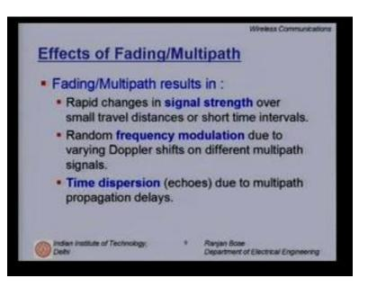
Now in this slide, let us look at the effects of fading and multipath. In literature, many times you will see the word multipath fading being used together. Fading and multipath results in rapid changes in the signal strength over small travel distances or small time intervals. Random frequency modulation occurs due to varying Doppler shifts on different multipath signals.
