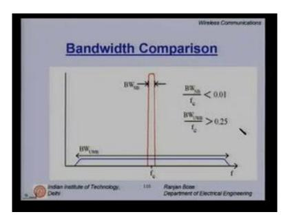
Just a bandwidth comparison. In the red is a typical narrow band system. Large power, very narrow band as opposed to R ultra-wideband system. It is extremely wide band but very low power and here the bandwidth divided by the centre frequency. It should exceed 0.25 - the 25% constraint.
