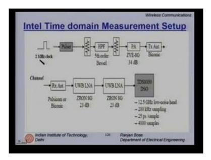
The measurement set up is as follows. As we mentioned, the 2 MHz clock is used to pulse it. Then they have a high pass  $5^{th}$  order Bessel filter and then after amplification, they send it through a bi-conical transmitter antenna. At the received antenna, they have first a low noise amplifier and then finally their measurement setup. This is the Intel time domain measurement setup.
