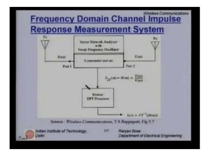
Here we learnt that we need to use a vector network analyzer which uses an S parameter test set to find out the S  $_{21}$  which is nothing but the transfer function given by H omega = Y omega divided by X omega. Clearly, if we know this complex transfer function, taking an inverse Fourier transform would give me the exact channel impulse response. In fact this is one of the more popular methods for indoor channel measurements.
