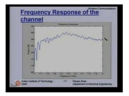
Just to give you a frequency domain response of the channel from 7 to 8 GHz. It is comes out like this. We are measuring the channel in the frequency domain. So this comes out directly.
