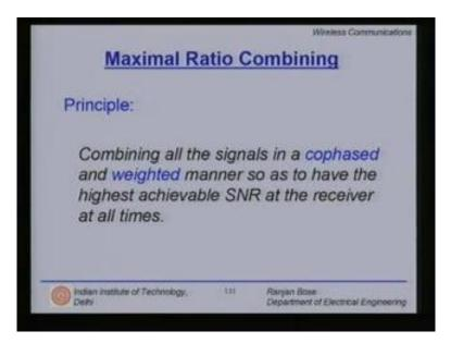
Let us look at the third technique which is also the more popular technique which is the maximal ratio combining method. What is the basic principle? You combine all the signals in a cophased and weighted manner so as to have the highest achievable SNR at the receiver at all times. In this sense it is optimal. So please note the two terms cophased and weighted.
