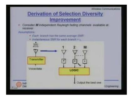
Here is a graphical representation for the selection diversity and suppose we have 1, 2 and so forth till M antenna and the transmitter transmits either a voice or a data digital format, here is the logic which outputs the best of the signals.
