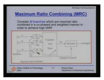
Again consider M branches which are maximal ratio combined in a cophased manner, so if you have these M branches here in the antenna then you have a method of adaptive control wherein you can choose the weights and the phases. So that you can weight it, cophase it and then pass it to the detector.
