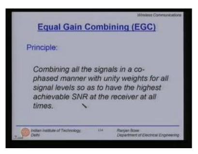
The fourth technique is a rather simple one; it is called the equal gain combining. What is the principle for this space diversity technique? We combine all the signals in a cophased manner with unity gained for all the signal levels. So that we have the highest achievable SNR at the receiver at all times, so here again we have to do a cophased addition but with unity weights.
