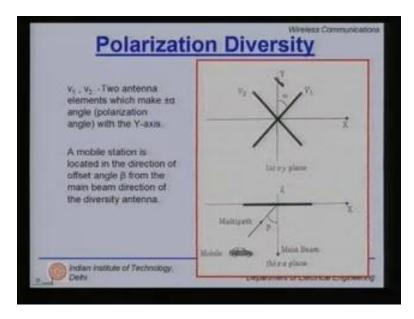
So here we have the two antenna elements which make an angle alpha here and we are trying to derive some results based on this angle alpha and a mobile is located in the direction of the offset angle beta shown here. So this is the main b, either is the offset angle beta and this is your mobile. So the antenna elements of the base station are also at an angle alpha with respect to the y axis.
