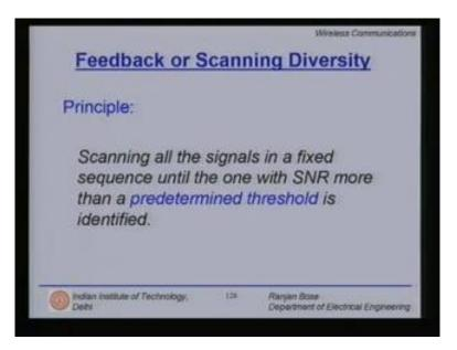
Let's talk about the second spatial diversity technique which is called the feedback or the scanning diversity. What is the basic principle? It scans all the signals in a fixed sequence until one with the SNR more than a predetermined threshold is identified. So we need to set a threshold before we start the operation and then we go into the scanning mode.
