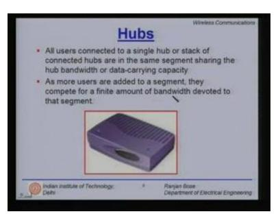
All users connected to a single hub or stack of connecting hubs are in the same segment sharing the hub bandwidth or data carrying capacity so the bandwidth is shared. As more users are added to a segment they compete for a finite amount of bandwidth, devoted to that segment. So you have to take this into account.
