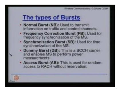
Now let us talk about the type of burst, when we talk about burst we are talking about data burst. We have the normal burst used to transmit information on traffic and control channels and we have frequency correction burst used for frequency synchronization of the mobile station. Then we have synchronization burst used for time synchronization of the mobile station, you can also have a dummy burst this is the BCCH carrier and enables mobile station to perform power measurements.
