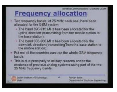
This is due principally military reasons and to existence of previous analog systems using part of the two 25 megahertz frequency bands. So this is what is in the standards depending upon individual countries part of the bands may be used. Now we know that a mix of FDMA and TDMA is being used in GSM.
