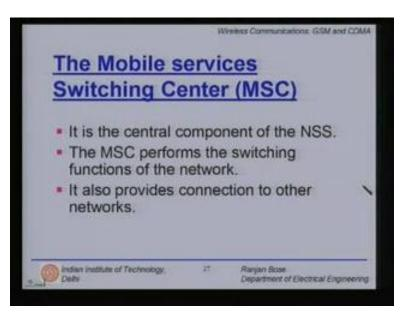
We now come to the mobile services switching center or MSC. It is the central component of the NSS. The mobile switching center performs the switching functions for the network. It also provides connections to the other networks primarily the PSTN or the public switched telephone network.
