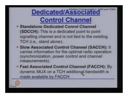
Talking about the dedicated and associated control channels we have a standalone dedicated control channel, the slow associated control channel, and fast associated control channels. These have different specified utilities and these are being listed here. The details can be found out from any standard textbook dealing with GSM. Now we move over to the modulation for GSM.
