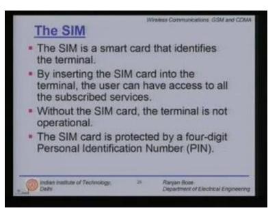
So you can take your SIM card move around inserted into any other terminal and start talking. Therefore a user can have access to its subscribed services in any terminal using the SIM card. Today more and more intelligence is being built in the SIM card, it has its own memory, it has its security features. So SIM card is becoming more and more important because it is fully loaded today with lot of features.
