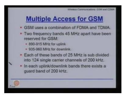
Now let us talk about multiple access for GSM. GSM uses a combination of FDMA and TDMA. The two frequency bands 45 megahertz apart have been reserved for GSM, one is the 890 to 915 megahertz for uplink and 935 to 960 megahertz for downlink. Each of these bands is of 25 megahertz is then further sub divided into 124 single carrier channels of 200 kilohertz. In each uplink or downlink bands there exists a guard band of 200 kilohertz.
