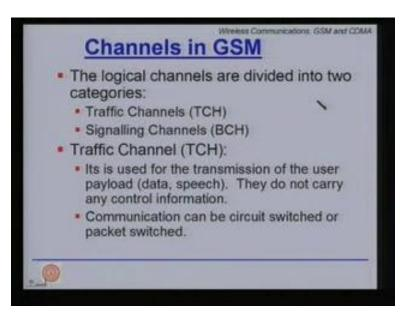
In the previous lectures we had talked about the public switched telephone networks where we saw the voice network and the signaling network, drawing parallel from that let's start talking about the various channels available in a GSM network. So the logical channels are divided into two categories traffic channels and signaling channels. We will denote the traffic channels as TCH and the signaling channel as BCH.
