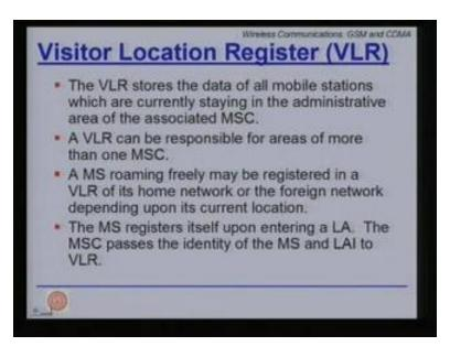
Now you have the visitor location register or VLR, the VLR stores the data of all mobile station which are currently staying in the administrative area of the associated MSC. A VLR can be responsible for areas of more than one MSC. A mobile station roaming freely may be registered in a VLR of its home network or the Foreign network depending upon its current location.
