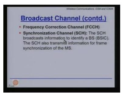
Now continuing with the broadcast channels we have the frequency correction channel or FCCH, the synchronization channel SCH which basically broadcast information to identify a base station. The synchronization channel also transmits information for frame synchronization which is important.
