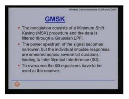
So GMSK modulation consists of minimum shift keying procedure and the data is then filtered through a Gaussian LPF. The power spectrum of the signal becomes narrower but the individual impulse response are smeared across several bit durations leading to some inter symbol interference. To overcome this ISI equalizers have to be used at the receiver.
