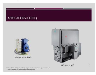
This picture shows an induction motor drive. This is an induction motor drive by ABB and this is just of a few kilowatts. So, inside this is the converter and the control for the induction motor. And this one is the picture of an AC motor drive by Siemens. And you can see from the picture itself, how much is the difference in the size as of megawatt level. So,
