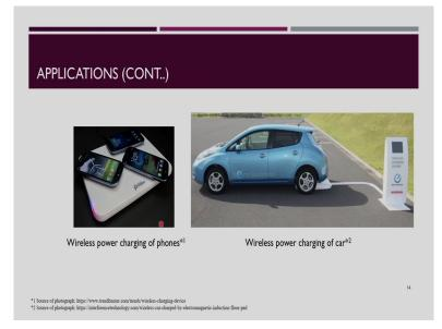
Another area of application is wireless power charging. So, this shows a wireless power charging of phone. So, in it, what you generally have is have the primary coil and, on this side, the secondary coil. So, it is like an air core transformer. It is used as a converter which
