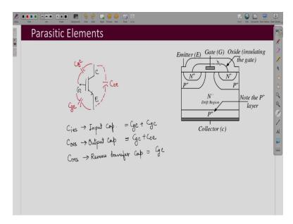
Now, what are the important parasitic elements associated with IGBTs we will be discussing only the important ones. So, this is IGBT and this is collector, emitter and gate terminal and then you have capacitances associated here between the collector and emitter which you can call it a  $C_{ce}$  and there is capacitance between these two which is gate to collector capacitance,  $C_{gc}$  and then there is capacitance between gate and emitter which is  $C_{ge}$ .
