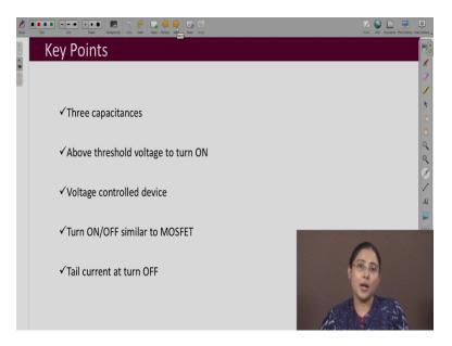
So, what are the key points of this lecture, three parasitic capacitances are important. They play an important role in the turn on and turn off of the IGBT and the voltage, gate to emitter voltage has to be above threshold voltage for it to turn on. And it is a voltage controlled device like MOSFET and turn on and turn off is similar to MOSFET. But there is tail current in IGBT which is not present in MOSFET and which makes IGBT relatively slower device then MOSFET. Thank you.
