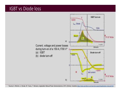
Now, one thing that I wanted to mention here is that, you have got an IGBT plus you have got an anti-parallel diode. So, you will need to do the loss calculations when you want to calculate the efficiency or you want to do the thermal design of converter. So, at that time you have to calculate all these switching losses and conduction losses of the IGBT as well as the diode.
