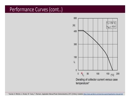
Then another important curve that may be provided is derating collector current  $I_c$  versus case temperature and as we expect as the temperature increases the maximum collector current allowed is going to decrease and that is what we observe here that there is a derating in the collector current.
