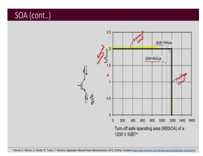
Then, let us look into turn off safe operating area, which is basically RBSOA. So, here you can see this is given twice of  $I_{C(nom)}$  the nominal current. Now, usually what happens is that IGBTs or all these power semiconductor devices, there is not just one chip inside the IGBT.
