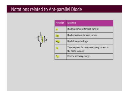
Then further there may be notations related to anti-parallel diode, this I had told you that most of the IGBTs the manufacturers make, they come with additional anti-parallel diode. So, this is that anti-parallel diode and so, the characteristics of this diode will also be provided.
