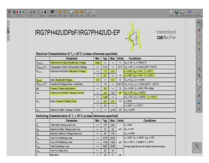
Then breakdown voltage, this 1200 V we have seen before. Then saturation voltage you can see typical is 1.7 and maximum is 2 V and at what conditions they have made these measurements, they are also given, so they change with these conditions, then what is the gate to emitter threshold voltage. So, that minimum is 3 V and maximum is 6 V.
