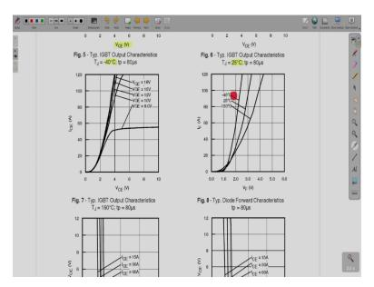
Then further this is given for your -40°C. So, this same is given for 25°C because this output characteristics changes with temperature. Then further the same output characteristics is
