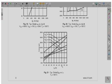
Then these are diode loss, and loss with respect to the diode current what the diode is going to carry. So basically, these are all diode characteristics that are provided by the manufacturer.
