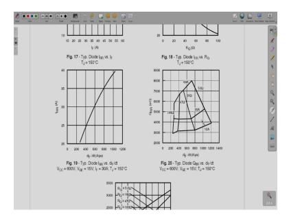
Then how this reversed recovery current  $I_{RR}$  changes with  $\frac{di}{dt}$ , this we had discussed when we discussed the diodes that these are also associated with the rate of change of current and so as  $\frac{di}{dt}$  changes, reverse recovery current is increasing as this is increasing. Then further it also gives reverse recovery charge of the diode versus rate of change of current and further you can see this for different resistance values and the limits are also given over here.
