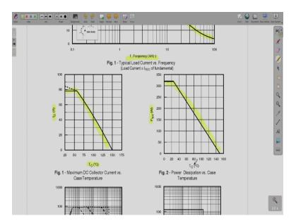
Further here this is collector current  $I_c$  versus case temperature. So, that is going to come down, this derating is going to happen as the temperature increases, then total power dissipation limit that is also going to decrease as these temperatures are going to increase.
