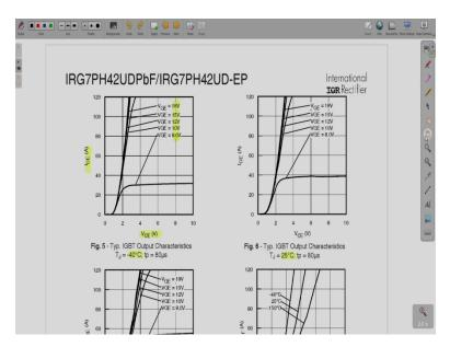
Further what you see is the output characteristics which is a graph between collector current and collector to emitter voltage and it changes with gate to emitter voltage. So, these are all the gate to emitter voltages that are applied and we can see here that it is above 12 V is what it goes into saturation and so, we should be applying more than 12 V.
