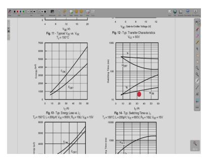
Then next is these losses with respect to collector current. So, you can see that this turn on losses they increase with collector current and turn off losses they also increase with collector current
