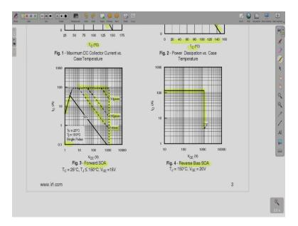
Then these are SOA curves. So, this one is basically provided by the saturation operation what is the current limit. You can see here the voltage is very small during that time and after that, this is current limit of the device, 100 A. This is the voltage limit of the device and then if we applied pulse for 1 ms, so, this is the power dissipation limit  $P_D$ .
