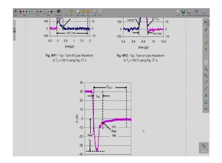
Then the manufacturer also has given different waveforms that they observed. So those results are provided here you can see that this is all diode reverse recovery waveform and then turn on loss waveform and turn off loss waveform this is what the manufacturer has provided.
