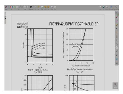
Further the same characteristics that we just saw is provided for maximum junction temperature 150°C. Then this is forward transconductance. So, this you can see that it is between collector current and gate to emitter voltage. So, this is where the collector current starts to increase. So, this is where threshold voltage is going to be. And these are given for two different temperatures.
