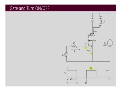
So, now, this is gate to source voltage  $v_{GS}$  which appears across the MOSFET. Now, here what we see is that form this time  $t_0$  to  $t_1$  for this time period the voltage first increases and it reaches to the threshold voltage  $V_{th}$  and at that time the voltage across the MOSFET does not change it is  $V_{dc}$  and the current through the MOSFET also does not increase it is equal to  $i_{DS}$  and we had seen that this time period is called as the delay time.
