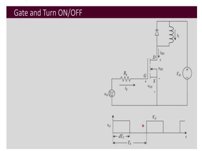
To understand that, let us first look into the turn on and turn off process of MOSFET and as we had seen before turn on and turn off process of MOSFET and IGBT are similar. So, we can take either of them and understand and the same applies for IGBT also. So, here there is a MOSFET and this is the gate circuit.
