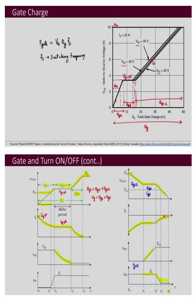
So now, what is the  $P_{gate}$  equal to?  $P_{gate}$  we can find out from this kind of graphs. This we have seen before also when we discussed the devices, this is gate charge versus gate to source voltage. And this is similar to this kind of graph that we see here, instead of time this voltage can also be plotted with respect to the charge.
