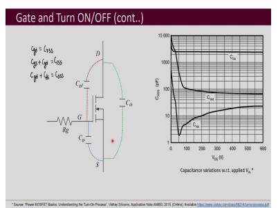
So, now, also recall that MOSFET has these three capacitances associated with it, parasitic capacitances one is gate to drain capacitance, then is gate to source capacitance and drain to source capacitance. Further, you have to recall that this gate to drain we have renamed it as  $C_{rss}$ , which is reverse transfer capacitance, then  $C_{gs}$  gate to source plus gate to drain that forms input capacitance  $C_{iss}$  and  $C_{gd}$  plus  $C_{ds}$  that forms output capacitance  $C_{oss}$ .
