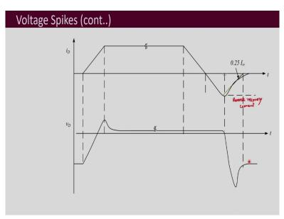
So, to some extent, we had discussed this when we discussed your turn ON and turn OFF characteristics of the devices of diodes and MOSFETs and IGBTs, now you have to recall this is the switching characteristics of the diode. We had seen this turn ON characteristics in the turn OFF and at that time I had told you it is the turn OFF which is more a problem then your turn ON and hear it turn OFF of the diode what happens is that you have this reverse recovery current.
