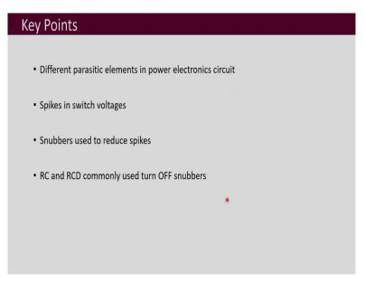
So, what are the key points of this lecture? What we discussed here is that the different parasitic elements present in power electronic circuits and they lead to spikes in switch voltages and that may damage the device. So, to reduce that we use a snubbers and the widely used to turn OFF snubbers, RC snubbers and RCD snubbers. Thank you.
