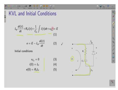
To analyze this RC circuit, we will apply KVL. So, here if you apply KVL in this part.
