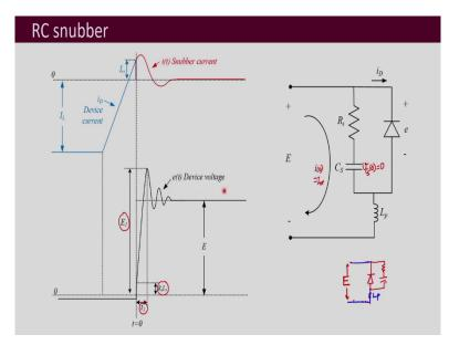
To analyze RC's snubbers I have taken this circuit. So, what it basically is that that we using this snubber design for this diode. So, in a circuit you have will have the diode connected and it may be connected to any part and there whatever the diode the voltage it is supposed to block that is your E and across the diode you will be connecting this RC and then it is close enough so, that we do not have to take into account any parasitic inductance here.
