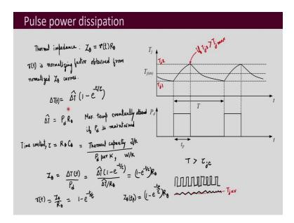
This graph shows that the power dissipation is in the form of pulses and the frequency of these pulses is small enough. This time period T is much large as compared to the time constant of the junction to case material. Let us say that the temperature was over here initially before this power dissipation pulse. So, as the power dissipation  $(P_d)$  takes place, the junction temperature increases and it reaches to another temperature.
