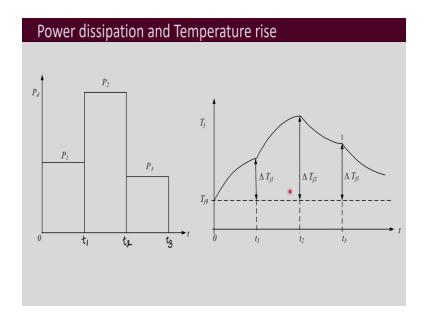
Now, power dissipation always need not be in form of just pulse, single pulse or repetitive pulse. It may be having different shapes. In these kind of different pulses for various values of power dissipation here, the power dissipation is assumed by  $P_1$ . The time duration is  $t_1$ , then till time  $t_2$  the power dissipation level changes and it has the value of  $P_2$ . Then further for another time up till  $t_3$  the power dissipation that takes place is  $P_3$ .
