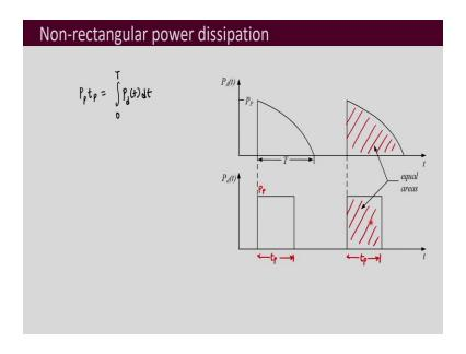
Now always it may not be in the form of rectangular pulses. The power dissipation may be of various different types of the shape. The power dissipation, you can plot and what you obtain may be very different. For example, it is shown here. Let us say the power dissipation is of this form which is taking place for this time period T and the peak is  $P_P$  and then it slowly reduces in this nature.
