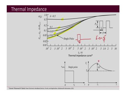
So, this is the nature of those graphs which are provided by manufacturers. So, here you can see that this one is the thermal impedance normalized and it is divided by the thermal resistance that means, this is the curve of  $r(t_p)$ . Over here this is the x axis, where the duration of the pulse  $t_p$  is given. Then, the thermal impedance for different values of  $t_p$  is provided over here.
