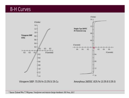
Now, depending on the material, BH curves can be very different, and there are different manufacturers of magnetic materials. They make the magnetic materials from different composition of different elements and based on it, obtained BH curve also is different. Now, here this is this material vitroperm 500 F. This is the name of that material and this has the composition, which is 73.5% Fe, 15.5% Si and 1% Cu.
