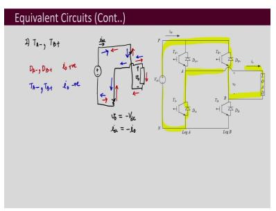
Next, see the second equivalent circuit for the second switching combination, which is the other two diagonal devices  $T_{A-}$  and  $T_{B+}$ . Now, let us say that this is the direction of the current. So, this transistor is on. So, if this transistor is on, the current is positive and it flows like this. It has to be conducted by the diode, it comes like this and then this device is on, so this also has to be carried by this diode.
