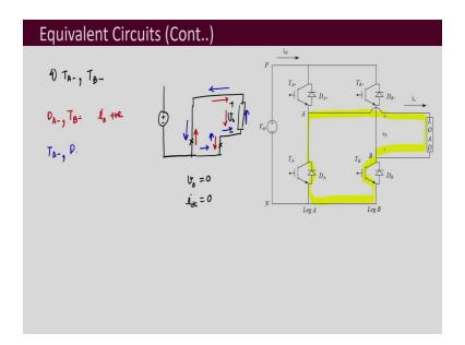
Now, the 4th one or 4th combination is  $T_{A-}$  and  $T_{B-}$ , where the lower two switches are being on. At that time, we observe here that the path will be like this. This is the circuit, and the path is going to be followed. So, let us draw the equivalent circuit again. So, the equivalent circuit will look like this.
