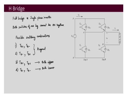
So, this is the circuit of H bridge converter. You see here that it has got four IGBTs. Now, 4 MOSFETs may also be there. It depends on the application. Here, I have shown four IGBTs and then there are 4 anti-parallel diodes. So,  $T_{A_+}$  and  $T_{A_-}$  has been named as the upper one and the lower one respectively. These two connected together are called as the Leg *A*.
