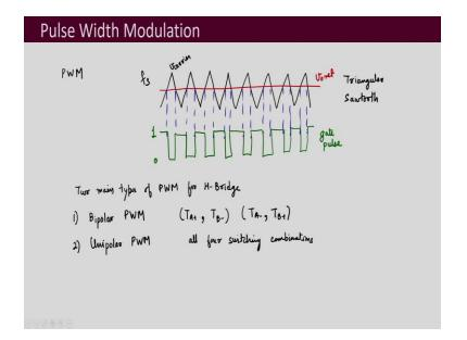
Now, you should be already familiar with the term pulse width modulation. In short, it is also called as PWM. So, what is PWM basically? Here is a carrier signal. This kind of a carrier signal which may be triangular in nature, or sometimes sawtooth. This has that frequency, which  $(f_s)$  is equal to the switching frequency. It is compared with a reference. Let us say this is the reference called as  $v_{oref}$  and we can call this as  $v_{carrier}$  and then these are compared.
