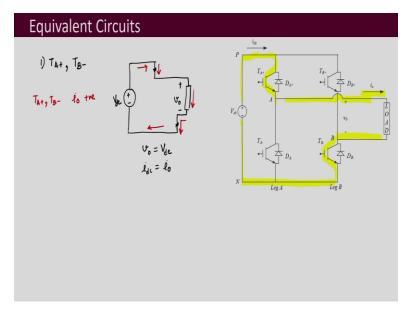
So, let us take the first one which is  $T_{A_+}$  and  $T_{B_-}$  being on together. So, here when this is shorted,  $T_{A_+}$  and  $T_{B_-}$  can be shorted. Now, the diode may also be conducting. We will see when the diode conducts and when the transistor conducts. But, to draw the equivalent circuit we can consider these as shorted, because we are considering it to be ideal.
