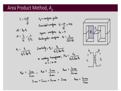
To design transformers again, I will show you the area product method. More or less the method is same, but there are some small differences. So, let us look into the equations for area product method. So, if we have a transformer and on the primary side the voltage is  $V_1$  and on the secondary side the voltage is  $V_2$  and the current over here is  $I_1$  and on the secondary side it is  $I_2$ .
