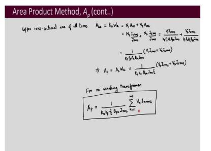
So, the total cross-sectional area or we can say that the total copper cross-sectional area of all turns will be given as
