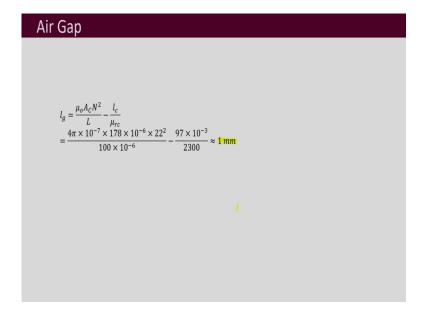
Then for the air gap again you have the equation for calculating this, you substitute all the values there in the air gap and you obtain that.
