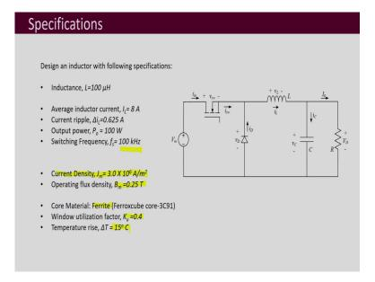
Now, let us take an example of inductor design. So, we need to design an inductor for a buck converter. Let us say that we have to design the inductance for  $100 \ \mu H$ . The average inductor current for that particular converter is 8 A and the ripple allowed is 0.625 A. Output power that means, the total output power here is  $100 \ W$  and the switching frequency chosen is  $100 \ kHz$ .
