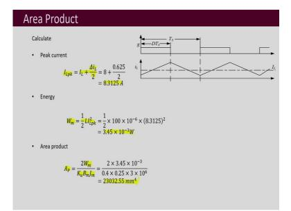
So, what do we do? We first calculate the area product and for that what we have to do? We have to first calculate the peak current. So, you know the equation to calculate the peak current. So, you substitute here and you obtain that this is the value of the peak current.
