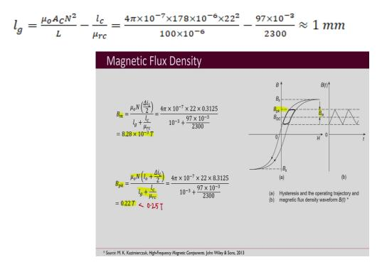
Now, let us do some checking whatever we have designed. We obtain the air gap length, we obtained the number of turns, the gauge of the wire, and also we selected the core. So, we calculate the  $B_m$ . So, what is  $B_m$ ? You know that  $B_m$  is this much of the flux density. So, you have the equation for that and you substitute again all the values. That will be
