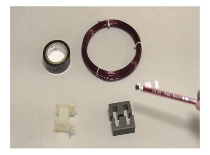
As per the area product calculation, the selected core is EE ferrite core which is made by Ferrox cube. The dimension of this core is
