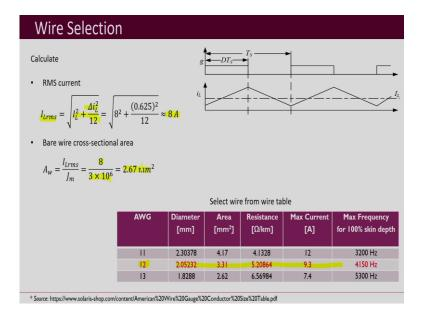
Then next step is to do calculations for the wire selection. So, for that you have to calculate the RMS of the current. So, that has been done here using this equation and approximately 8 A is again obtained. So, if the ripple is small, RMS current is going to be close to the average current.
