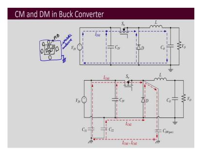
Now, what is this common mode and differential mode? How is it actually taking place inside of an electronic converter? So, let us take an example of buck converter. So, this is the buck converter circuit that you are familiar with and then this is the reference. This symbol right now over here is the reference. Do not assume that this is earth, this is a reference.
