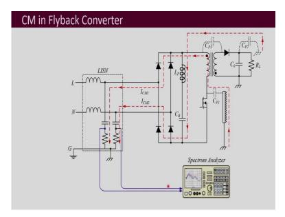
If we see how is the common mode current arising, for that we have to see the different points where capacitors is getting formed between any point and the ground. So, we observe here that this point definitely will have some capacitance with respect to the chassis ground. In between these two primary and secondary also there will be some parasitic capacitance and further these devices will also have the parasitic capacitance with respect to the chassis ground because of the heat sink.
