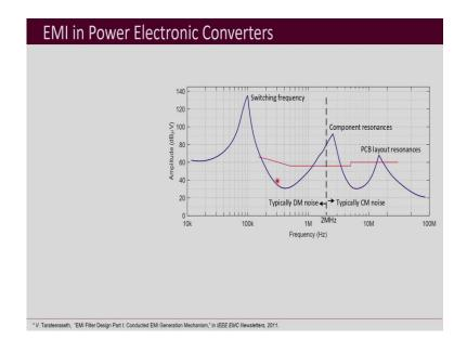
So, now this common mode noise and differential mode noise have different frequency range. Usually common mode noise is obtained above 2 MHz of frequency and the frequency components in common mode noise is observed. This common mode noise is more because of the component resonance. That means the parasitic capacitances and other parasitics are present in the devices. We saw that MOSFET's and diodes have got their capacitances. So, some of these capacitances are with respect to the ground.
