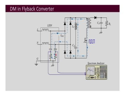
So, let us see that this is some other converter also. So, this is example of a flyback converter. Here, this part is flyback converter. So, here you have a simple rectifier. Now, here this LISN is drawn. We have seen LISN before. It is the equipment which is used for measurement of conducted EMI and this is somewhat like a filter circuit.
