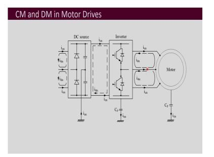
Then CM and DM noise are present in all power electronic converters and in motor drives also. So, I showed you how it is present in converters, the motors that we use in the electric drives. When you are having motors, they further add up to some of the sources of common mode noise because you might have heard about bearing currents and all that. So, that is like common mode voltage which gets formed and that affects the motor performance.
