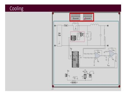
Then further, what is there is your cooling section that comprises of your heat sinks fans or if you have liquid cooling the cold plates and whatever the cooling arrangement further the accessories that are required for the cooling, so, that is your cooling section that will be there new converter.
