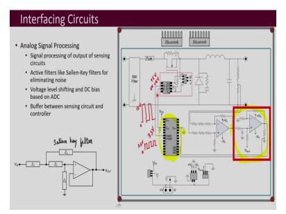
Then your interfacing circuit. Now, what is an interfacing circuit? Interfacing means you have to interface between two different sections and usually sensed output and the controller and you have to interface between the two that means you have to match the voltages in between them. Means your output of the sensor is let us say giving with respect to your 15 V and your controller accepts voltages of the range of 3.3 V.
