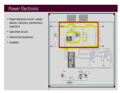
So, first of all is the power electronics section. So, power electronics section means that is your, this, this box that I have drawn here, that one that contains your power electronic circuits. A power electronic circuit here is this thing, this one, this buck converter familiar circuit, that is
