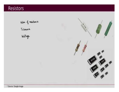
Resistors are required in power electronic circuits for sensing and control circuits. There are different types of resistors available.
