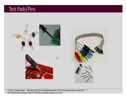
Then other types of components which are used are the miscellaneous components like the test pins here you can see that this is a test pin to which this probe is attached to if you want to see the voltage over here. So, these kinds of through-hole test pins maybe there are SMD test pins that may also be a place for some time.
