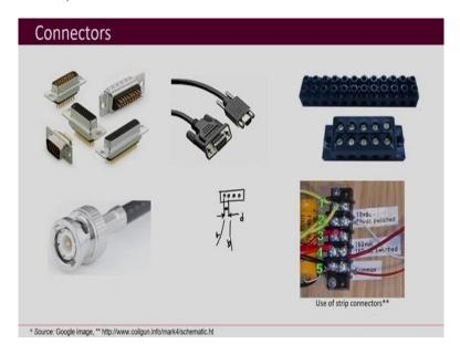
The next type of connector is your these D sub connectors and these are also for your transmitting signals they are used both analog and digital both types of signals may be taken over when you have more sensitive signals which means you want to protect more from noise, then these type of D sub connectors can be used. And then further if you have radio frequency signals to be carried then this type of connectors are used which are your BNC connectors.
