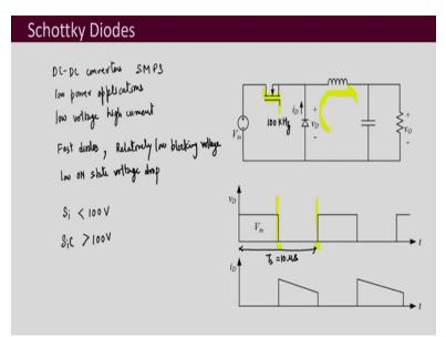
Now, next let us look into the application of DC to DC converters. So, DC to DC converters, let us say we are using it for SMPS applications. So, those are mostly low power applications and the power requirements, the power levels are usually up to few hundred watts and there they are many times called as low Voltage high current applications.
