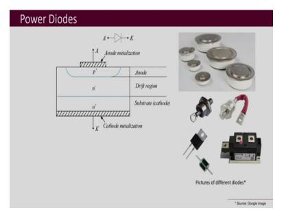
Now, let us begin with power diodes. So, this is the physical structure of the power diode, where you have a p+ region and then you will have n- and n+ region and then you have the anode and the cathode and this is the symbol of the diode, which you must be familiar with.
