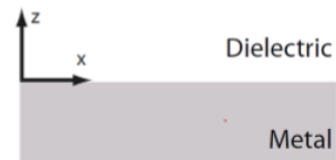
Figure: Geometry for SPP propagation at a single interface between a metal and a dielectric.
