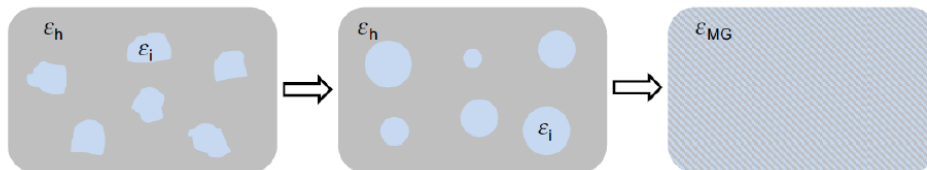
Figure: Illustration of Maxwell Garnett homogenization.
