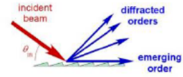
Figure: Rayleigh anomaly: A sharp intensity variation and related exclusively to the emergence of the diffracted beam.
